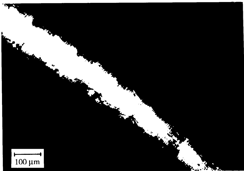
Figure 2. The extrudate melt fracture from anisotropic cellulose solution viewed under crossed polar microscope.
